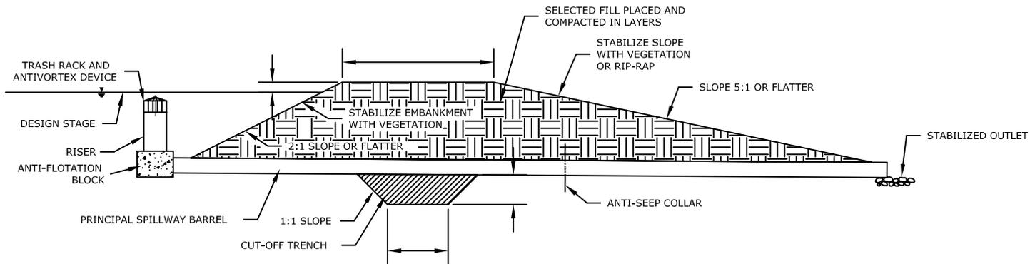
SECTION THROUGH EMBANKMENT AND CONTROLS - CLASS 1 BASIN
