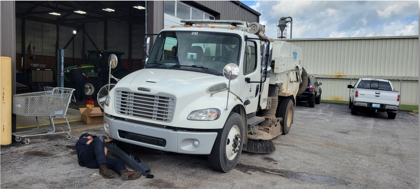
Figure 11-Mr. Nick Updegraff installs a new magnetic pick-up bar on a sweeper at Fleet (7 Aug)
