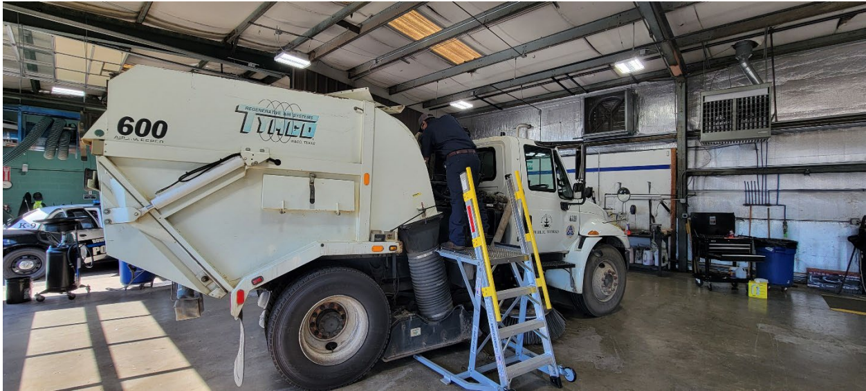
Figure 13-Service Technician Nick Updegraff services our 2006 street sweeper. The unit has 88K miles and 11,573 engine hours (11 June)
