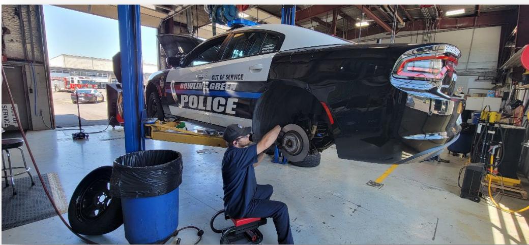
Figure 16- Service Technician Trevor Noble replaces the brakes on a police cruiser (13 June)
