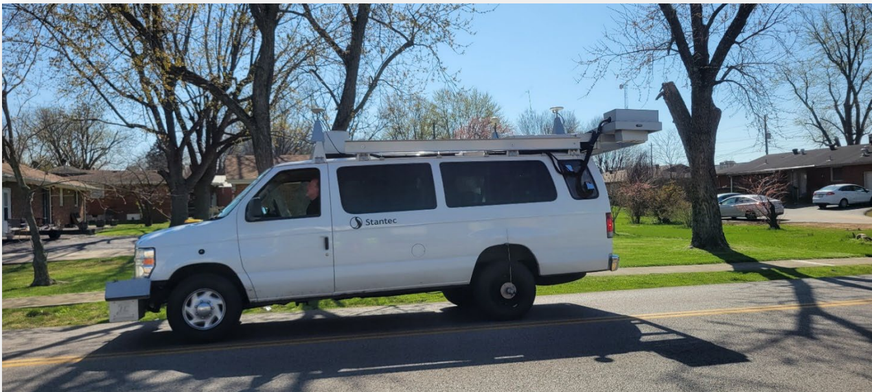
Figure 8-A Stantec vehicle collects road condition data on Creason St (20 March). City-wide collection data will be used to inform next year’s Overlay.
