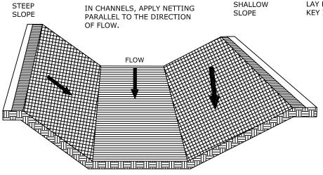
LAY FROM BOTTOM UP W/4" LAP. KEY IN AT TOP OF SLOPE/BERM.
