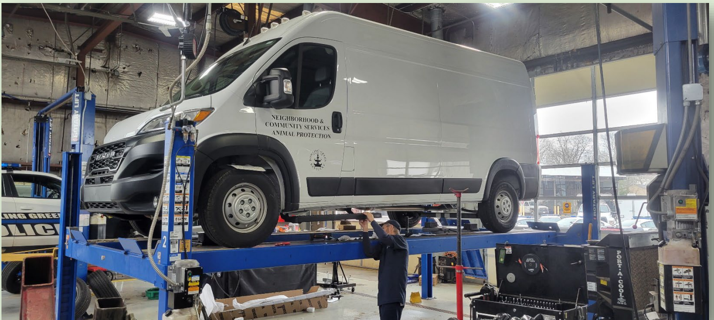
Figure 1- Service Technician Keith Patton installs access steps on the new Animal Protection van at Fleet. The vehicle will also be wrapped by a vendor with new markings to increase public awareness. (9 Feb)
