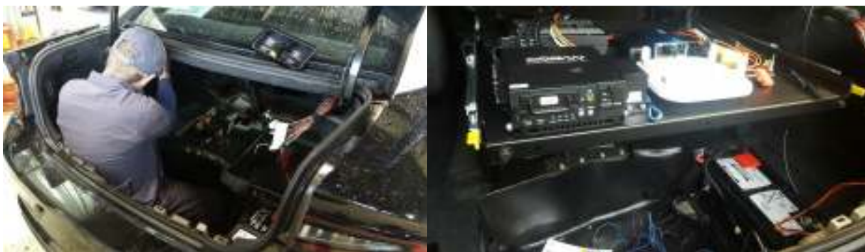
Technician installing rear wiring and required IT components
