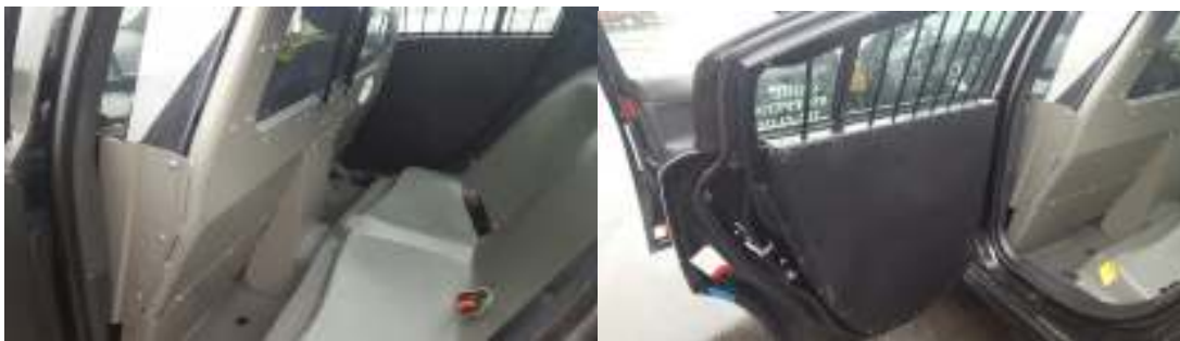
Rear seat and cage after full outfitting
